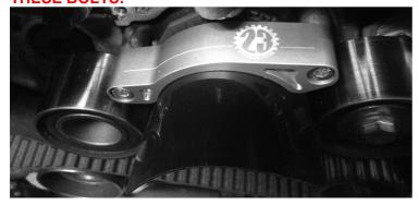
Step 5) Remove the Company23 Timing Belt Guide Spacer Tool.
