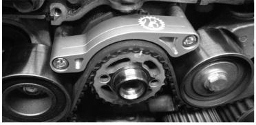
Step 4) Insert the supplied Company23 Timing Belt Guide Spacer Tool between the timing belt and guide. Press down on the belt guide so that there is an even gap around the belt that is the thickness of the spacer tool. Tighten the bolts to 9.8Nm (1.0kgf-m, 7.2 ft-lb) using a 5mm socket. WARNING: DO NOT OVERTIGHTEN THESE BOLTS!
