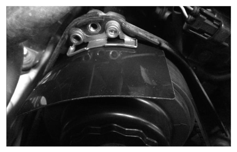
Step 8) Remove the Company23 Timing Belt Guide Spacer Tool.
