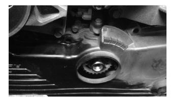
Step 2) Remove the timing belt guides. On manual transmission cars, you will need to remove the factory belt guide using a 10mm socket. If you are changing the timing belt at the same time, follow those steps now. (See Company23 Cam Lock Tool #506 Manual for more)
